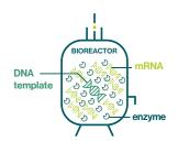
To produce mRNA, the DNA template is transcribed into mRNA in a bioreactor. This enzyme-based process is known as in-vitro transcription (IVT). More than 500 mRNA strands can be produced with a single DNA template obtained from a plasmid.
